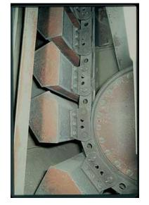
177.80 MM Pitch Bucket Elevator Chain with integral K5 attachments at every outer link.
